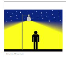
Full cut-off lighting directs light down and to the sides as needed.
